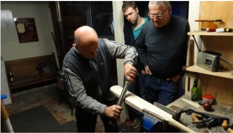
Boning the bat edges using the steel bar.
