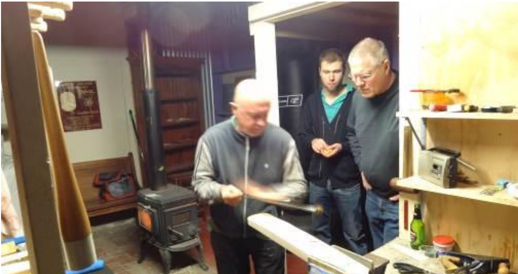
Shaping the back of the bat using the large spoke shave.
