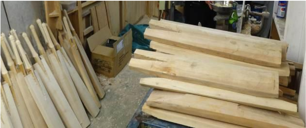
Partially machined willow blanks (right), and with the handles glued in (left).
