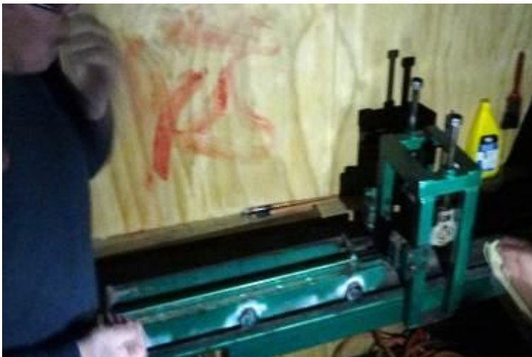
Lachlan's custom made rolling machine. The bat is placed face up on the carriage on the left, and fed under the rollers on the right.
