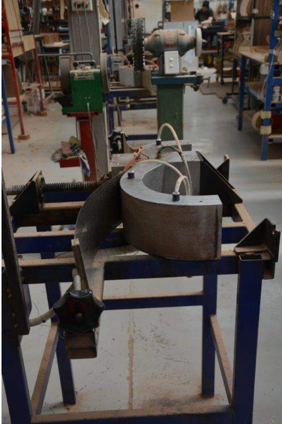
The bending jig used for jumbo guitar bodies.
