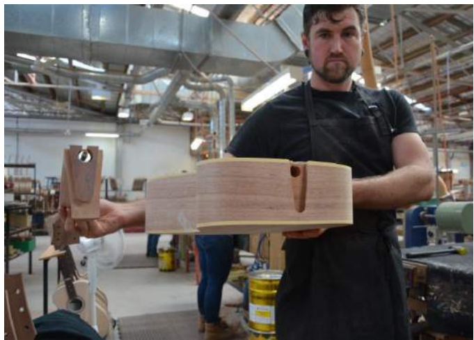
A unique dovetail method for fitting the neck to the body.
