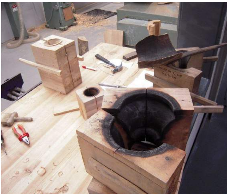
Wooden casting moulds, before and after use.
