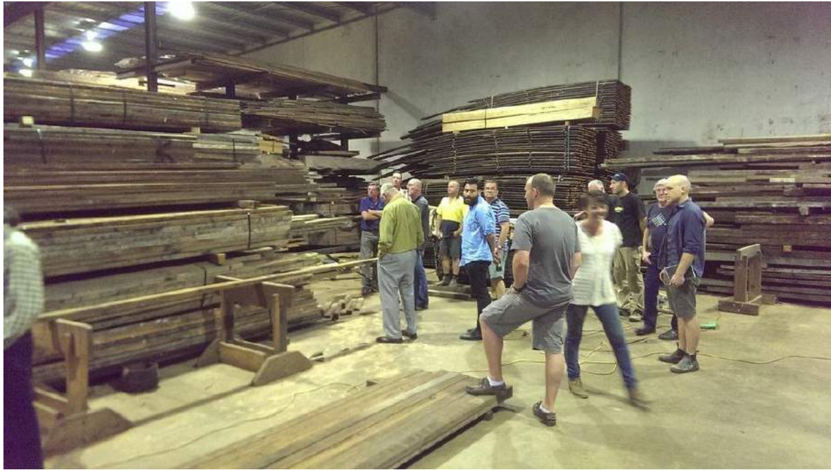
De-nailed and re-sawn timber stacks. These boards will be subsequently dressed and machined into flooring, wall cladding, bench tops and custom made furniture.
