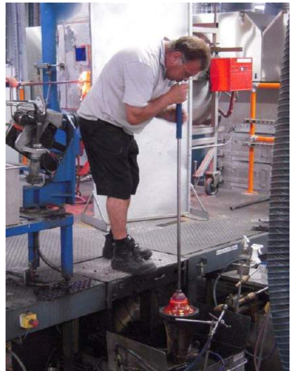
Blowing a vase into a wooden mould.
