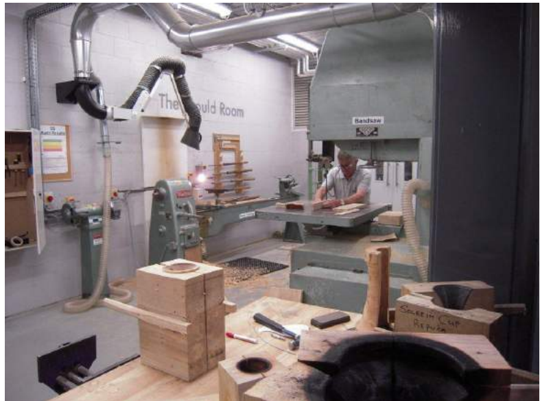
The wood workshop, with the usual range of equipment, table saw, bandsaw, lathe and dust extract system.
