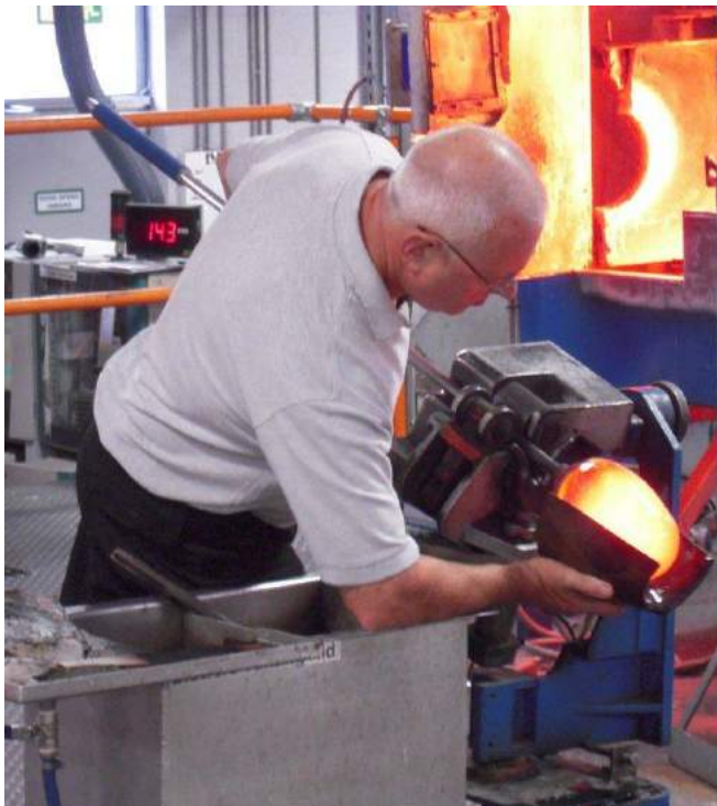
Initial shaping of a vase using a wooden shaping tool.
