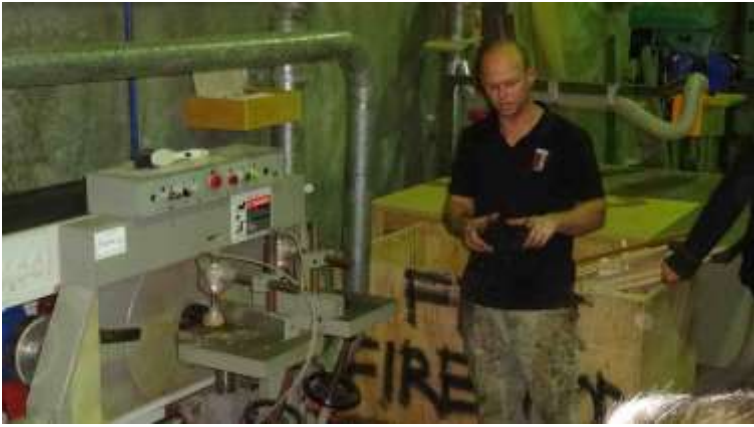
Christian explains setting up the tenon cutting machine.
