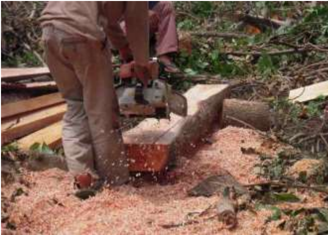
Photo 6 Cutting a guideline using the toe of the saw.
