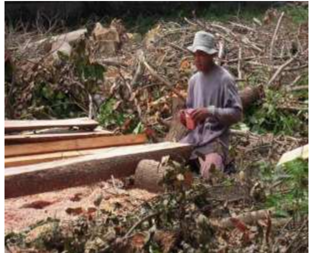
Photo 3 Using a string line in preparation for cutting.
